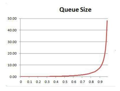
By plotting this function we can see that the average queue size remains low while utilization is up to 0.8, then rises sharply and goes to infinity. We can understand this intuitively by thinking about our computer's CPU: when its utilization is low, it responds instantly to our inputs, but when a background task pushes its utilization close to 100%, the computer becomes frustratingly slow to respond to every click.
